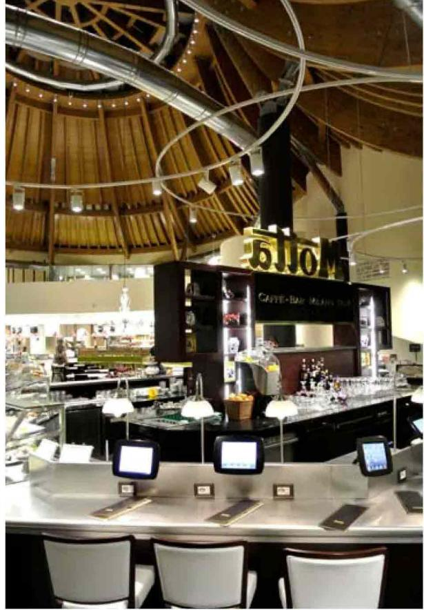
With a strong focus on eco-friendly, recyclable building materials, **Holzbau** constructed the exposed framework from PEFC-certified, glued laminate timber. The layout is remarkable for the complete lack of architectural barriers, allowing free passage between different areas and services distributed over a total area of approximately 2,500 m<sup>2</sup>. Among the companies involved in the construction: **Marazzi** for the ceramics and **iGuzzini** for the LED lighting.
